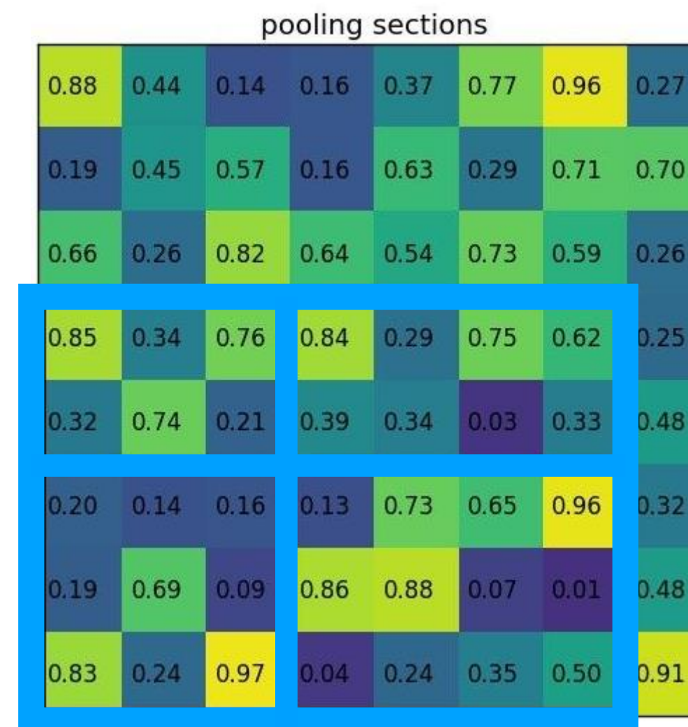
(1) Grid up proposal box into a fixed number of cells (eg 4 cells)
